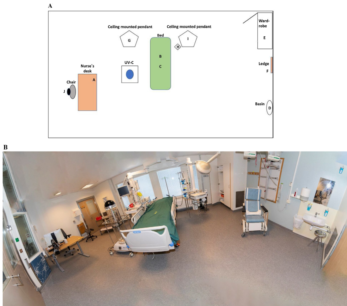
Fig. 1 – A) Room overview. Positions of indicators and radiometer (A) on the nurse's desk, (B) on the bed, (C) under the bed, (D) in the basin, (E) in the wardrobe, (F) on the ledge on the wall, (G) in the drawer of the left ceiling mounted pendant, (H) on the infusion pump, (I) on the drawing surface of the right ceiling mounted pendant, and (J) behind the desk chair. B) Panorama picture of the room in the burn ICU. Photo: Tony Lif.
